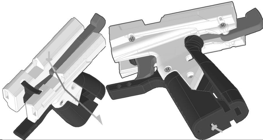
Tie a knot in the free end of the elastic cord and fish the opposite free end through the holes in the sear, trigger, and Griddle prints.
