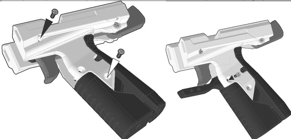
Drive two 4-40 screws into the holes where indicated. Repeat for the opposite side. Slide the Tguard print into the front of the assembly and secure with two 4-40 screws.
