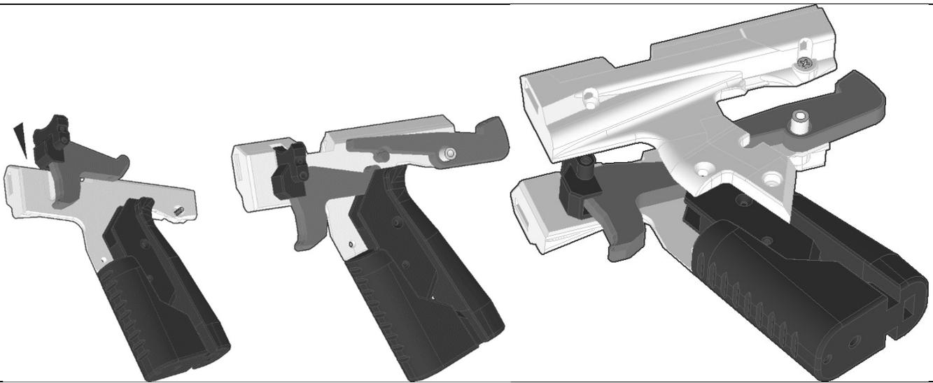
Place a plastic spacer into the center hole of the Sear print. Sandwich the Sear, Griddle, and GripB prints inbetween the GripRight and GripLeft prints, placing the screws you drove into the GripLeft and Grip Right prints into the center hole of the plastic spacer. The GripB print should fit into the slots in the GripLeft and GripRight prints.
