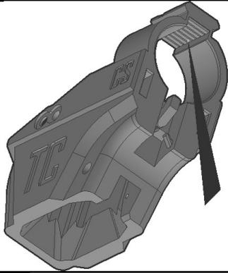
Inspect the indicated area of the Lower print for sagging filament strands. Test fit an aluminum bar inside the open rectangular slot. If obstructed by strands, use a round needle file in the indicated area to sand them down until the aluminum bar slides freely.
