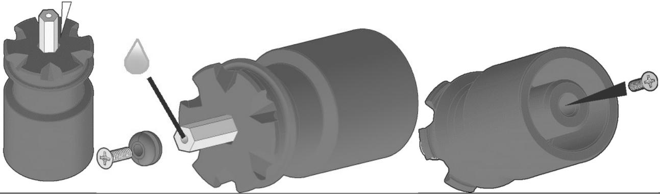
Push the long hex standoff into the front of the Plunger print. You may need to use a hammer to tap it into place until it bottoms out in the socket.
