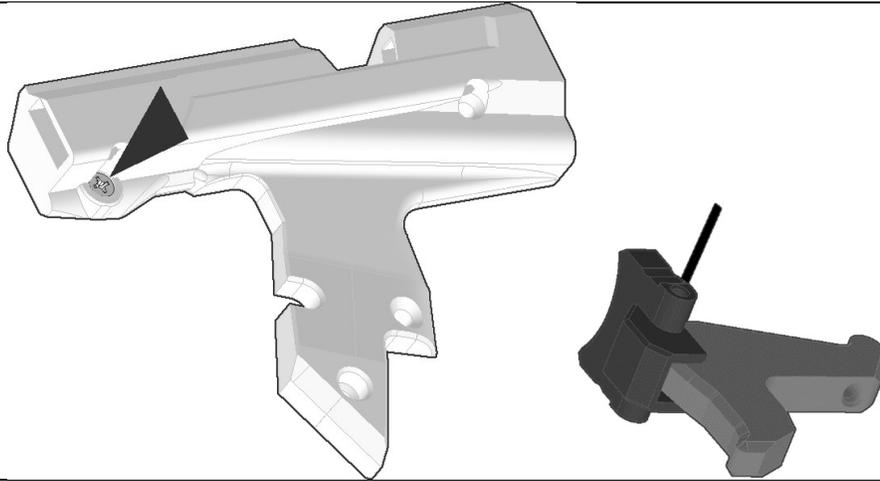
Drive a 4-40 screw into the GripRight print where indicated until it bottoms out. Repeat for the GripLeft print. Line up the hole in the Trigger print with the through hole in the GripB print. Force a short pin through both until centered.
