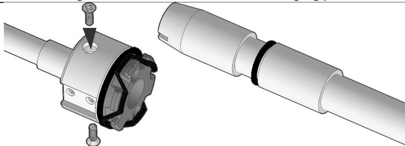
Drive a screw into each side of the RamF print until it clamps against the Ramrod Core.
