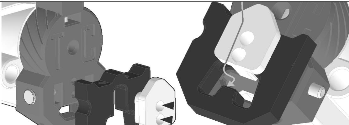
To add the optional collapsible stock slide the washer print into the slot in the Latch. Then line up the holes in the Washer print with the holes in the back of the Butt print. Drive a 4-40 screw in through each hole. Fish some elastic cord in through the hole in the top of the Latch print, out the middle of it, then fish the free end into the hole inside the hoop of the Butt print.
