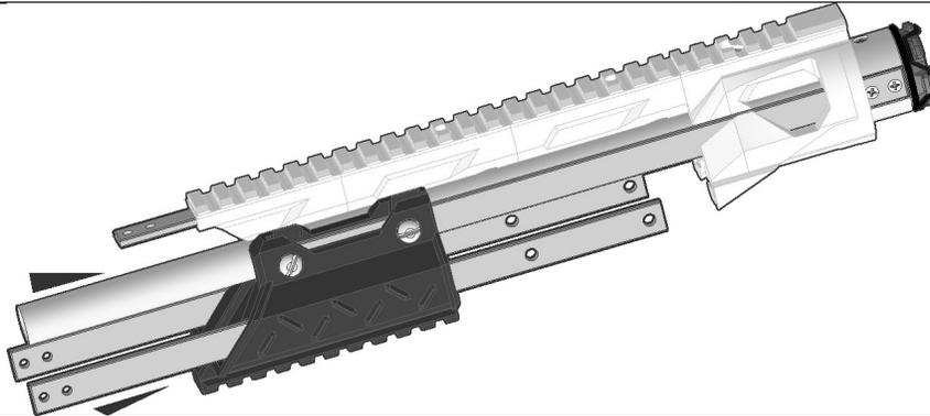
Slide the barrel in through the middle of the DOOM print and then into the socket in the front of the MagUpper print until it bottoms out.
