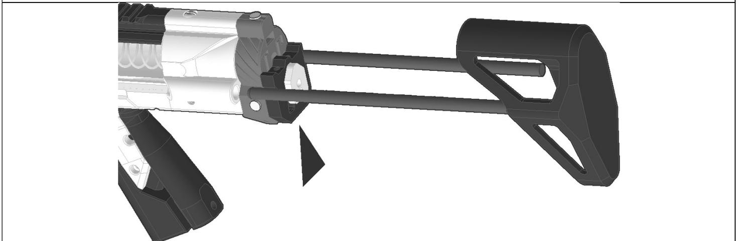
Push up on the Latch print from underneath, then slide the optional stock (custom or Worker PDW stock) into the holes in the Kiri print.
