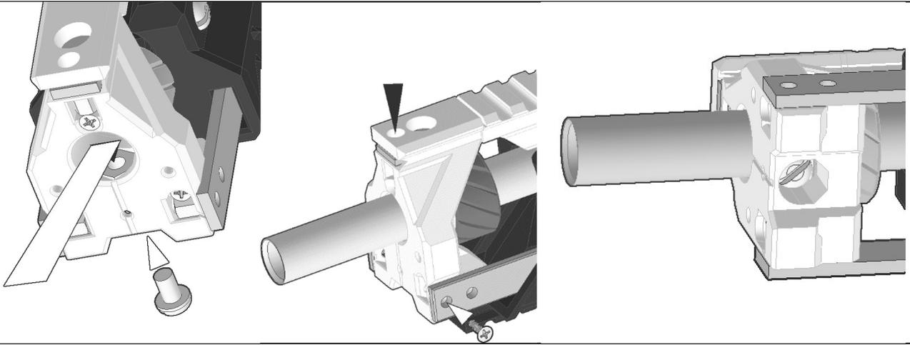
Put a hex nut into the slot inside the Muzz print, then drive a 10-32 screw into it from the hole in the underside of the print.
