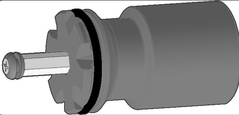
Add a 123 o-ring to the undercut of the Plunger print. Apply and spread some silicone oil onto the rubber grommet and o-ring.
