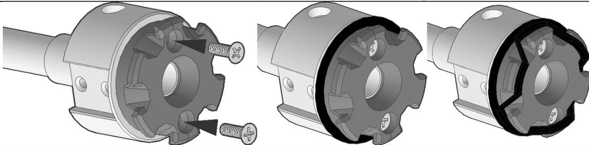
Drive two screws through the RamB print and into the RamF print until the two are clamped together.
