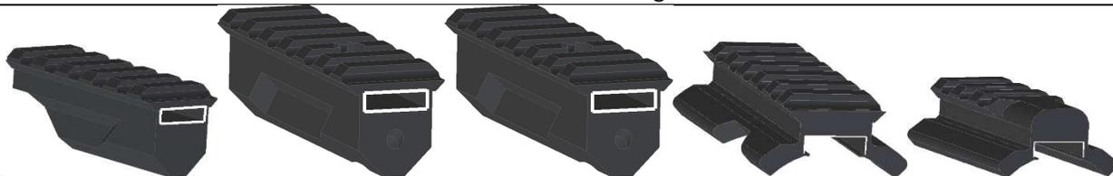
Use a sharp knife to deburr the edges of the rectangular holes in the prints shown above. Test fit the aluminum bars inside each, and repeat the deburring process if needed until the aluminum bar slides freely in each.
