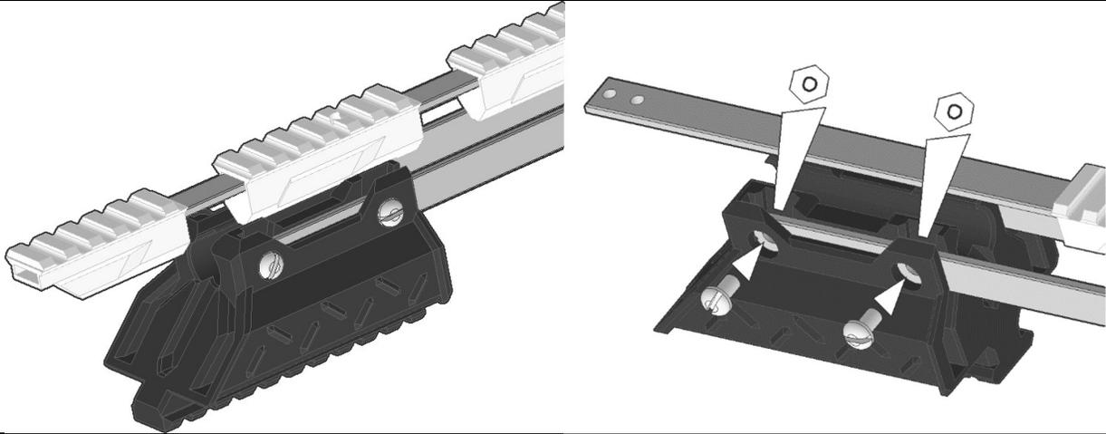
Slide the Doom4 Print onto the pair of Bolt Arms from the Ramrod assembly. Slide the next BS print and then the BSF print onto the upper Bolt Arm.
