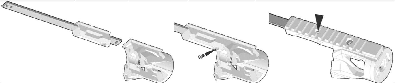
Slide a BS print over a Bolt arm piece as shown, then slide the Bolt arm into the slot in the front of the MagUpper print as shown until it bottoms out. Drive a 4-40 screw in through the angled hole in the underside of the BS print to secure it to the MagUpper print.
