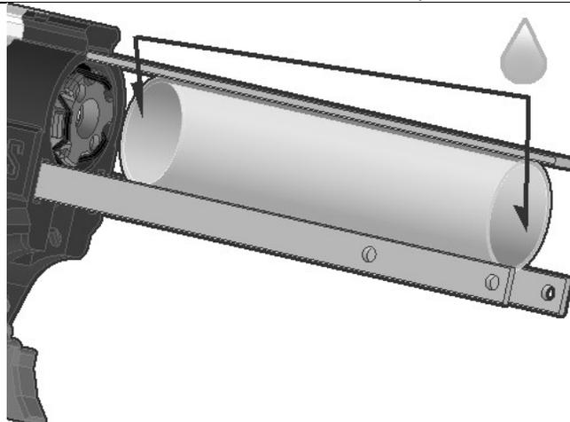
Apply some silicone oil to the inside of the plunger tube near both ends.
