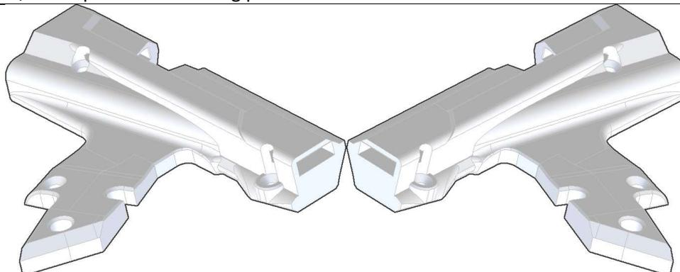
Use a small slotted screwdriver to check the inside of the rectangular slots in the grip side prints for loose or sagging printer filament strands. Test fit an aluminum bar inside each, and repeat the interior cleaning process until the aluminum bar slides freely in each.
