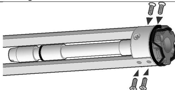
Line a BoltArm4 up to the slot in the side of the RamF print and drive two screws through the holes and into the RamF print until secure. Repeat for the opposite side.
