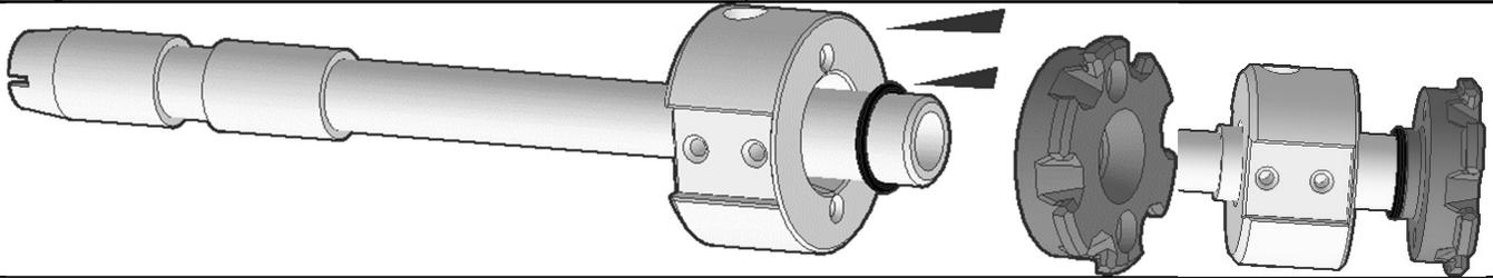
Slide the RamF print onto the back of the Ramrod Core.
