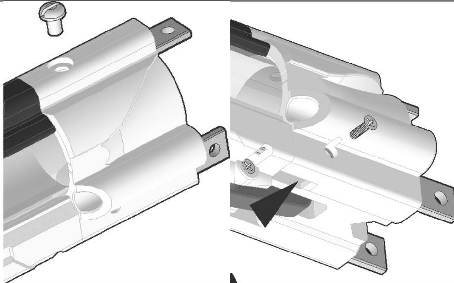
Line up the hole in the hex nut with the hole in the upper Bolt Arm, then drive a 10-32 screw in through the print and bolt arm until it drives into the hex nuts and clamps in place.
