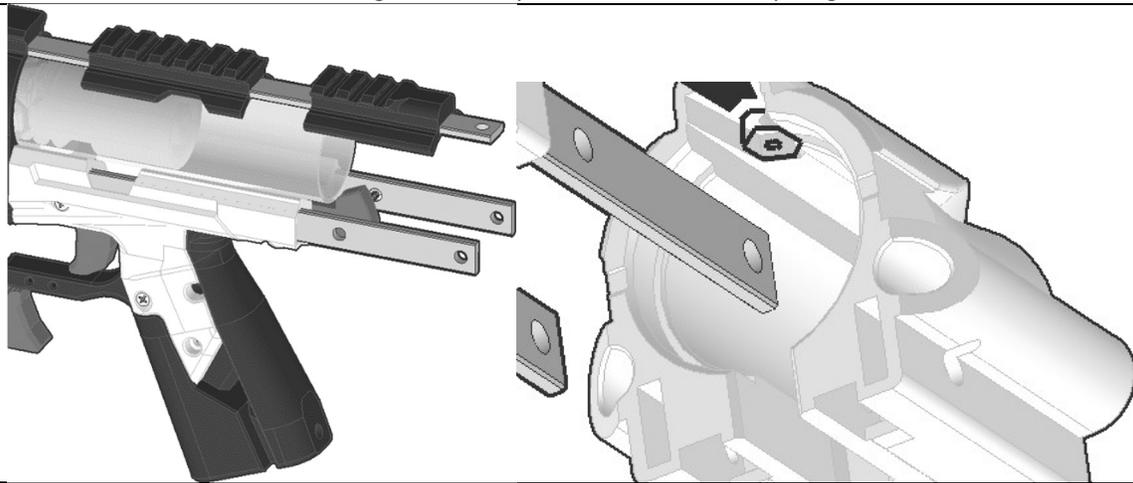
Slide the Rail1 and Rail2 prints onto the upper BoltArm4. These prints may need to be deburred at one end in order to fit.
