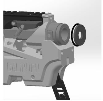
Add a 123 o-ring to the rear undercut of the Ramrod. Then remove the backing paper from the Shockpad and adhere it to the back of the Ramrod.
