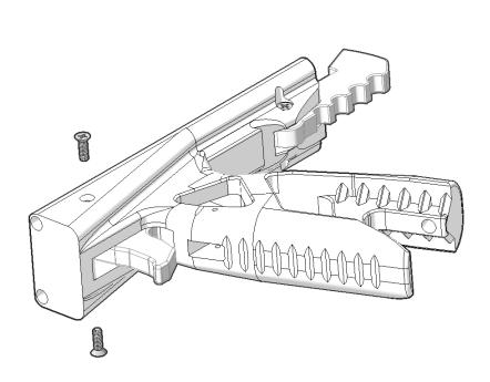
You can use a 4-40 short screw on each side of the grip to retain the Short Pin for the trigger.
