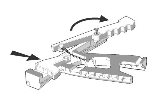
Fish the TRIGGER in through the front of the grip. You may need to pivot the SEAR back in order to get the TRIGGER in place. Once in place, the bump on the back of TRIGGER needs to sit underneath the front lip of the SEAR.
