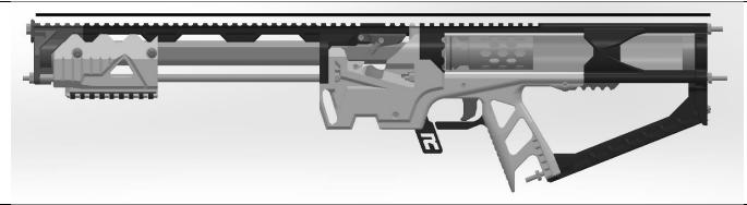
Check the top side of the assembly against a ruler or another flat surface. Adjust the tightness of the hex nuts at both ends of the blaster until the topside is as close to flat as possible. Also look down the top from the back and make sure that the assembly is straight from right-to-left. Adjust if it isn't.
