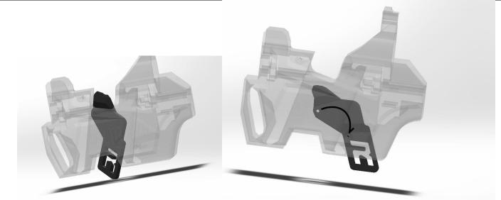
Slide the MagRelease up into the inside of the Magwell. Rotate it and then back it down into the slot in the back of the Magwell until the small hole in the MagRelease lines up with the small hole in the sides of the Magwell.
