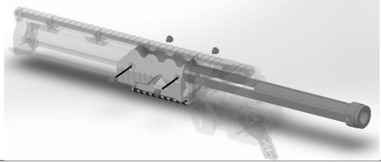
Slide the Boltarms and Foregrip together until the threaded holes line up with the holes in the Foregrip. Secure them together at the rear pair of holes using two short 10-32 screws. Repeat for the opposite side.
