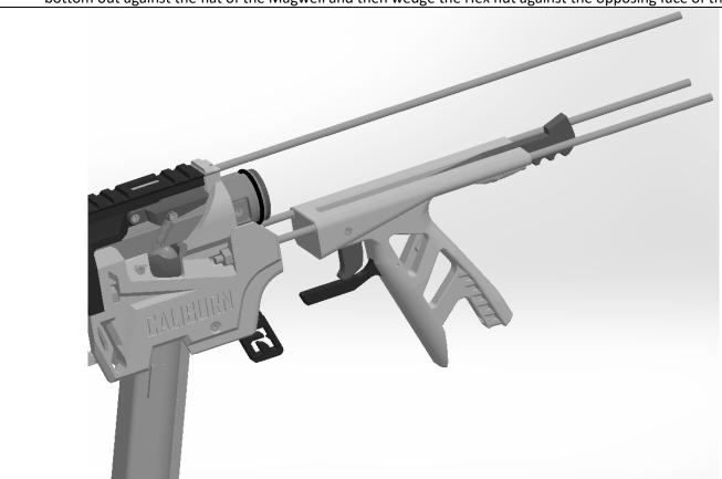
Slide the completed Grip assembly onto the 13" Threaded Rods.
