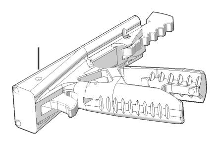
Slide a Short Pin in through the side of the grip and through the hole in the TRIGGER. You may need to use a 1/16" drill bit or another Short Pin and a hammer to lightly tap it through the trigger.
