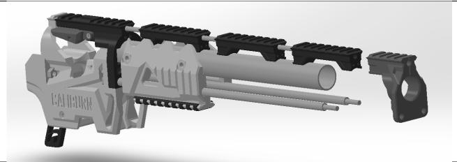
Slide the RailR segments onto the upper threaded rod, then slide the Muzzle onto the upper threaded rod, barrel, and lower threaded rods. You can optionally add one or two short pins between the DartJam, segments, and muzzle piece.
