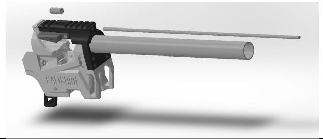
Add a coupling nut to the slot in the top of the DartJam piec. Screw a 14-inch length threaded rod into the DartJam from the top hole in the DartJam.
