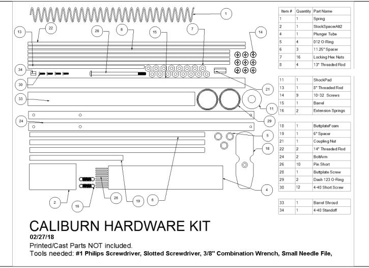
For most of the above hardware list the quantities are the MINIMUM required for assembly. Easily-lost items will have several spare and I typically include extras of the majority of the items. The quantity for Item #16 for this version of the Caliburn will need to be THREE, but having FOUR might be preferable.
