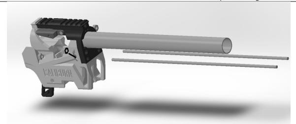
Slide a hex nut into the two slots where indicated . You may need to use a flat screwdriver to push them down to the bottom of the slots. Screw two 13-inch length threaded rods into those hex nuts from the front of the Magwell. If extra leverage is needed add an acorn nut to the opposite ends of the threaded rods so that you can use a wrench to tighten them into the hex nuts.
