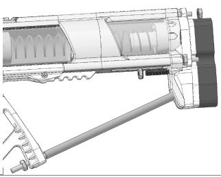
Add a hex nut to the exposed upper threaded rod and tighten it. Add a hex nut to the long screw and tighten it.
