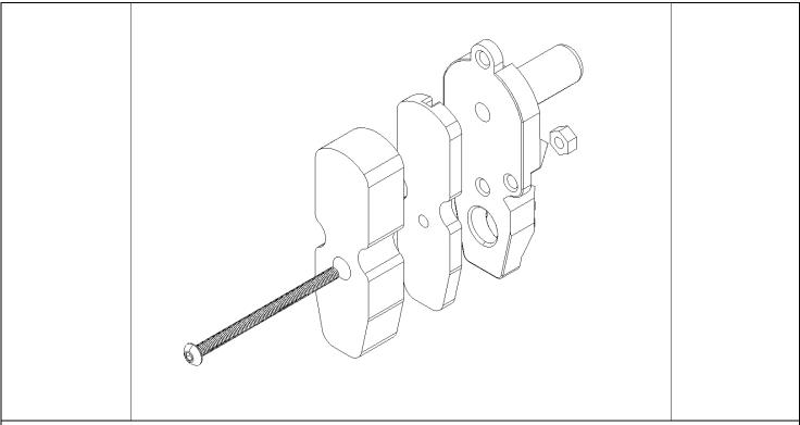
Adhere the Buttplate Foam to the Buttplate. Attach the Buttplate to "Back Butt" using the Long Screw and a Hex Nut. Set aside for later.
