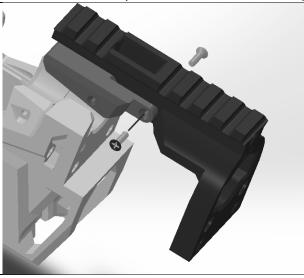
Attach the Tooth to the Dartjam by driving two 4-40 screws directly into the holes in the Tooth print. Make sure not to completely bottom out the screws in these holes as doing so might split the print.
