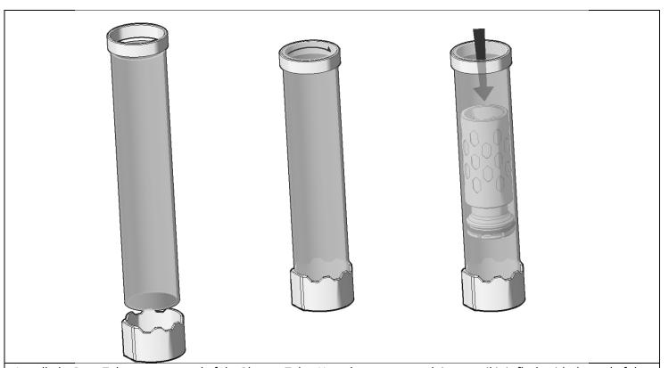
Installed a Ryan Tube onto one end of the Plunger Tube. Use a hammer to push it on until it is flush with the end of the tube. Install the Ring on the opposite end until it too is flush.
