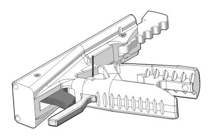
Slide the Tguard piece into the slot in the front of the Grip.
