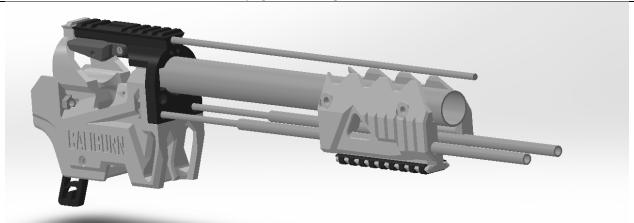
Slide two Nylon spacers onto the lower pair of threaded rods.
