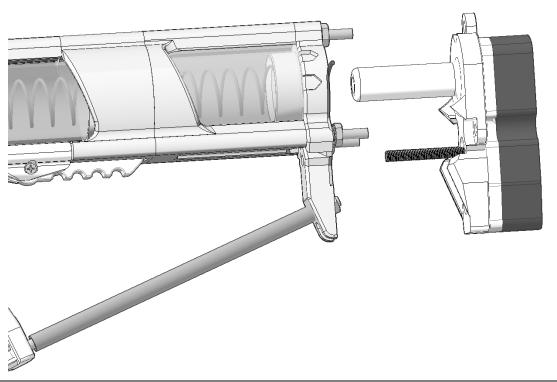
Align all of the Hex nuts parallel with the FrontButt itself so that they will engage correctly with the 12-point socket features in the ButtPlate.
