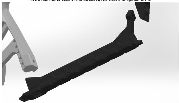
Wedge a nylon spacer or the printed stock spacer between the heel of the grip and the end of "FrontButt". You may need to file the sides of the little nub at the back of the printed stock spacer in order to get it to fit into the slot of the FrontButt piece.
