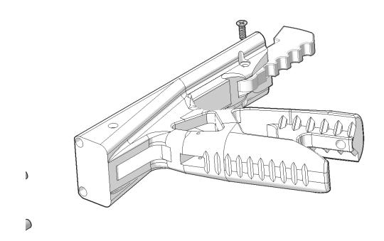
Use two short 4-40 screws to secure the standoff to the back of the grip.
