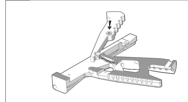
Insert the 4-40 standoff into the center hole of the SEAR and pivot it down towards the back of the grip.
