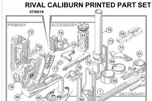
Note: Print layers should not be any larger than 300 microns. Parts were designed for PLA filament, but can be printed using ABS without issue. No support material is needed. Most of the parts should print to tolerance on their hole diameters, but results may vary so expect to have to touch up some of them with a round needle file
