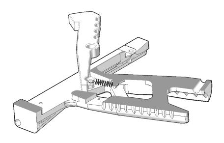
Add an extension spring to the peg on SEAR and use SEAR to fish the extension spring into the grip. Push the loop of the extension spring onto the hook inside of the grip.
