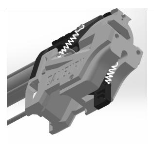
Drive a 4-40 screw halfway into the small hole in the side of the Tooth print. Hook one end of an extension spring to it, then the other end to the exposed screw in the side of the Magwell.
