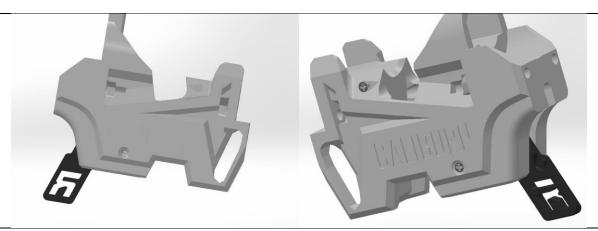
While holding the two up to a light, slide a short pin in through both. Drive a 4-40 screw into the small holes of the Magwell to close the hole off. Repeat with the opposite side of the Magwell while making sure that the short pin does not fall out. Drive another 4-40 screw halfway into the small hole further up the side of the Magwell.
