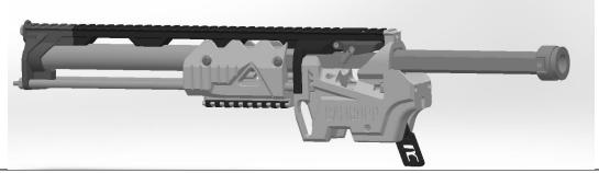
Slide the Foregrip forward and make sure the Ramrod is entering the Barrel during this action. If it isn't doing so smoothly, double-check its alignment. Tighten the hex nuts at the front of the assembly then re-check that the ramrod is still entering the barrel smoothly. You will need to adjust the hex nuts again if the Ramrod isn't cycling smoothly.
