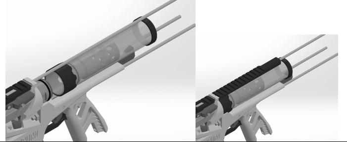
Hold down the trigger down and work the front end of the Plunger Tube assembly onto the back of the Ramrod O-Ring.
