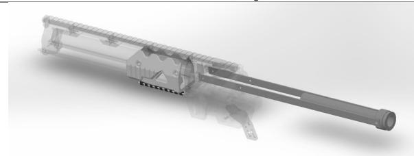
Slide the Bolt Assembly forward through the slots in the Magwell. You will need to pivot the Tooth part out of the way in order to do so.
