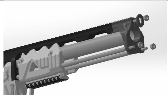
Add the RhopT to the upper threaded rod so that the knife-edge side is facing the Muzzle. Add a hex nut to each threaded rod and tighten each by hand only for now.
