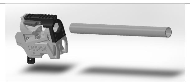
Check the fit of the Barrel inside the barrel hole of the Dartjam. If it does not fit you will need to touch up the inside with a round file. Install the barrel in the hole so that the back of it is flush with the lip on the Magwell and Dartjam.
