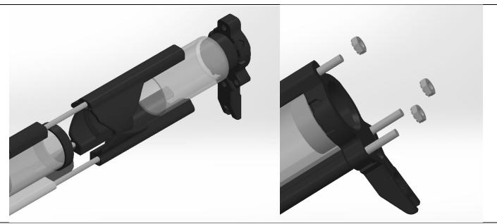
Slide the Stock\_Alt part onto all of the threaded rods.
