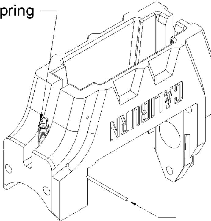
Insert a Pin through the MagWell and through the loop of an Extension Spring. You may need to use a pair of needle-nose pliers to get the pin centered. Once it is centered you can push or pry it towards the bottom of the magwell.
