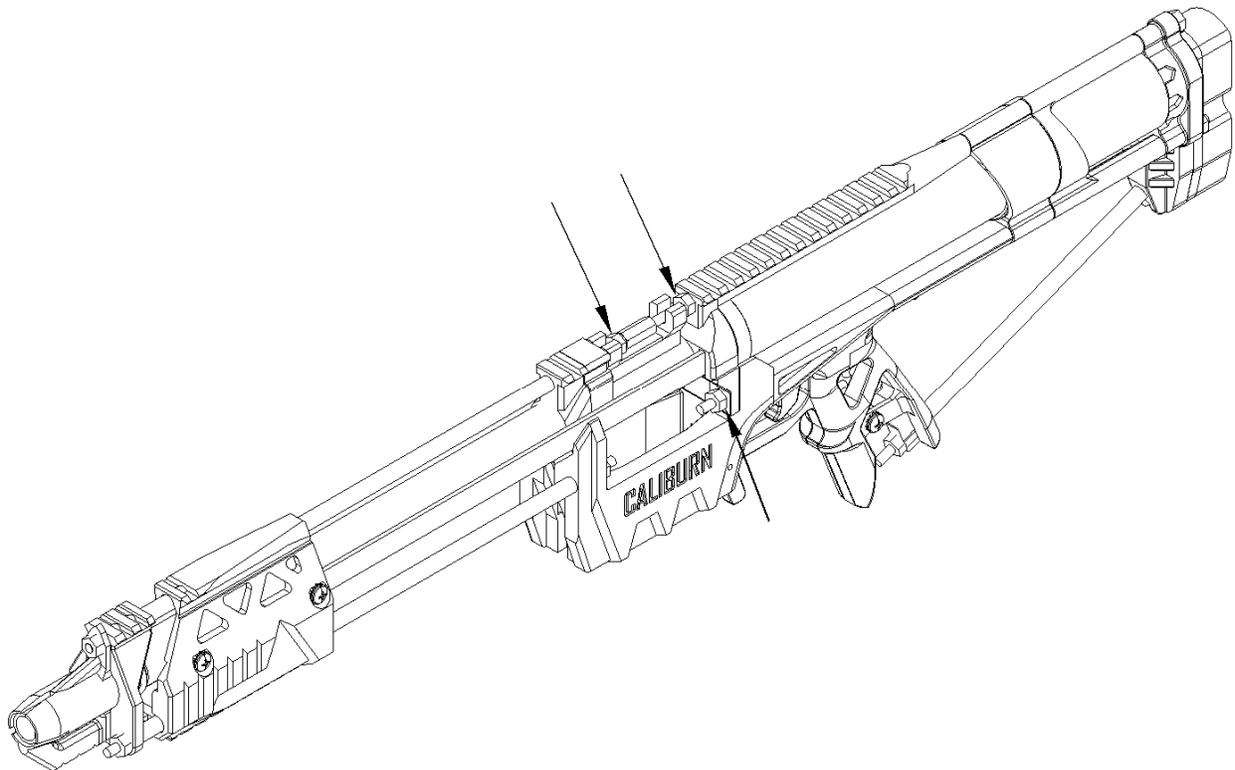
Tighten both of the lower Hex Nuts against Spreader until all of the components of the rear assembly are pulled together firmly. Tighten both Hex Nuts up top. One against the front tab of Jam, the other against Spreader.
