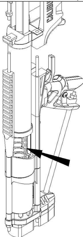
Rest the Buttplate against a chair or table and drop a Main Spring into the Stock. Carefully lower the Plunger Tube and Front Assembly over the Main Spring.
