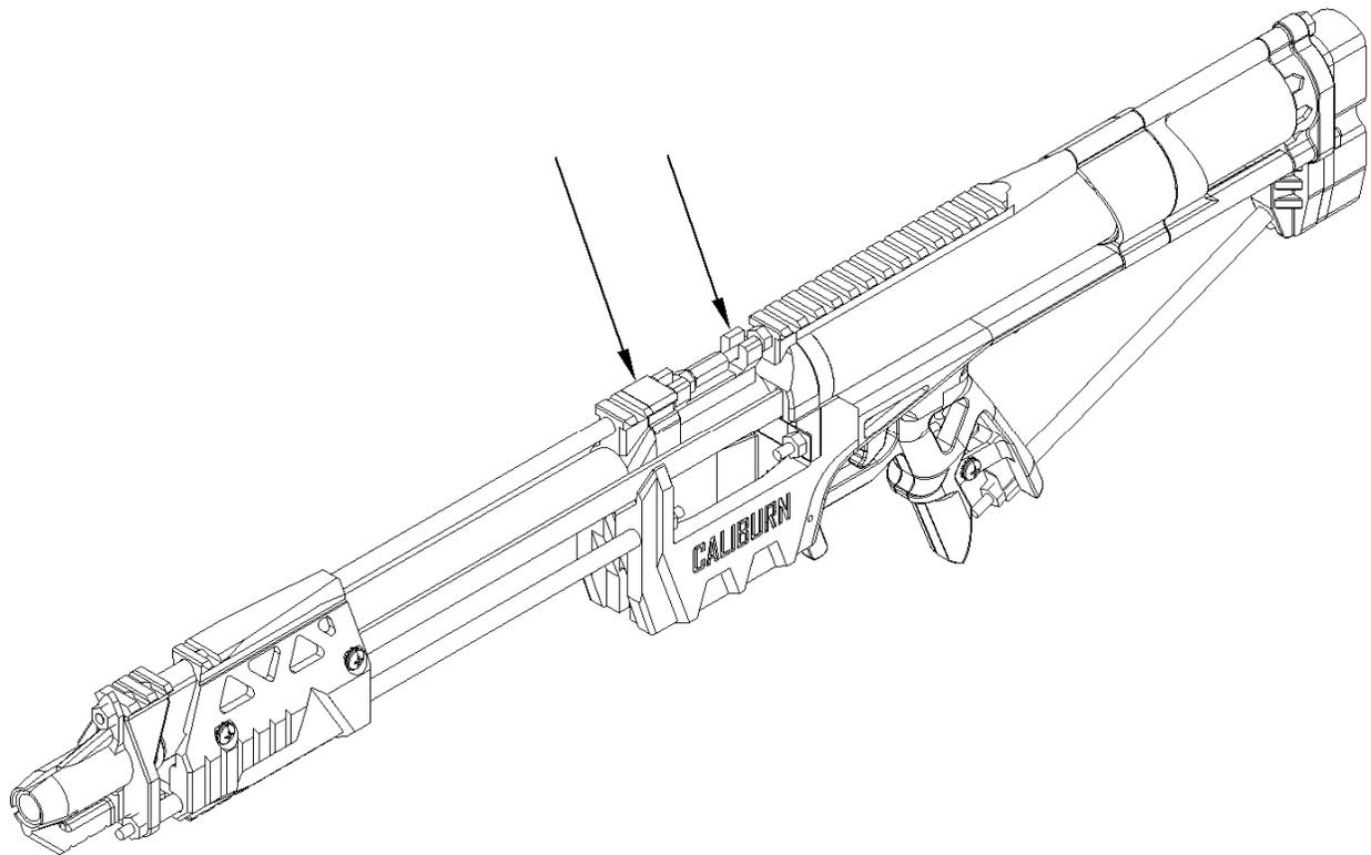
You will need to adjust the positioning of the upper 14" Threaded Rods for this next step, which is why they have not yet been tightened. Slide the Dart Guide onto the front 14" Threaded Rod from the top. Slide the Jam onto both from one side so that the front Hex Nut is behind the tab towards the front of the Blaster. Then rotate the Jam piece until it is oriented vertically.
