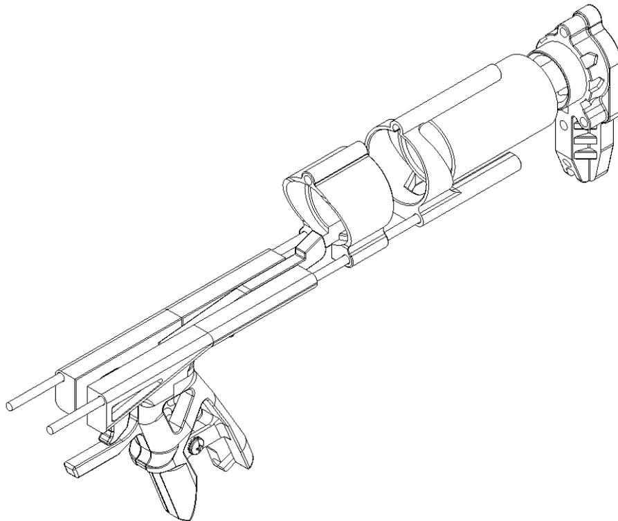
Slide the parts shown onto the 13" Threaded Rods. They include Stock\_Alt2, Ansuzalgiz2, Stock Spacer (clear), and the Butt assembly from earlier.
