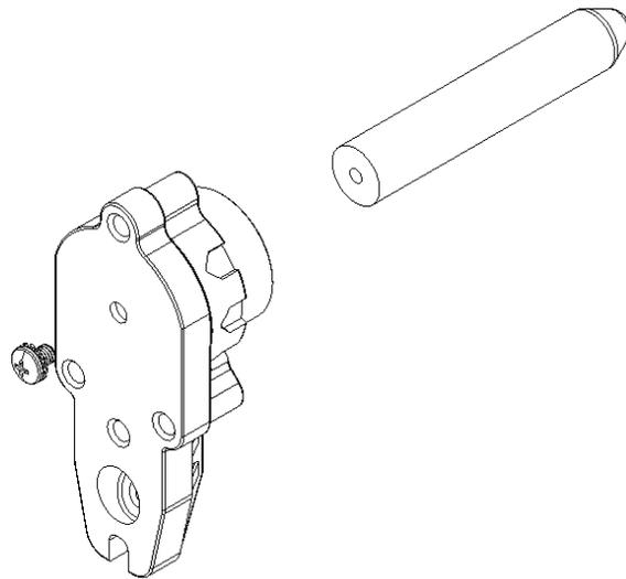
Attach the Stock Core to the Butt piece using a Short Screw.
