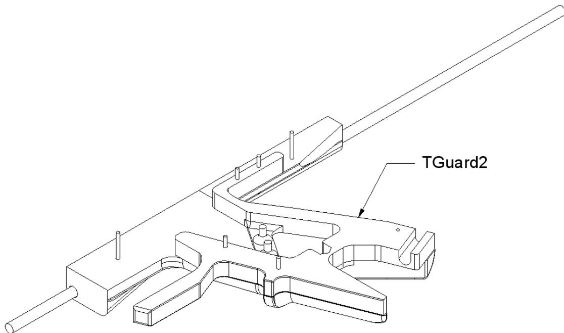
Slide TGuard2 onto the pins.
