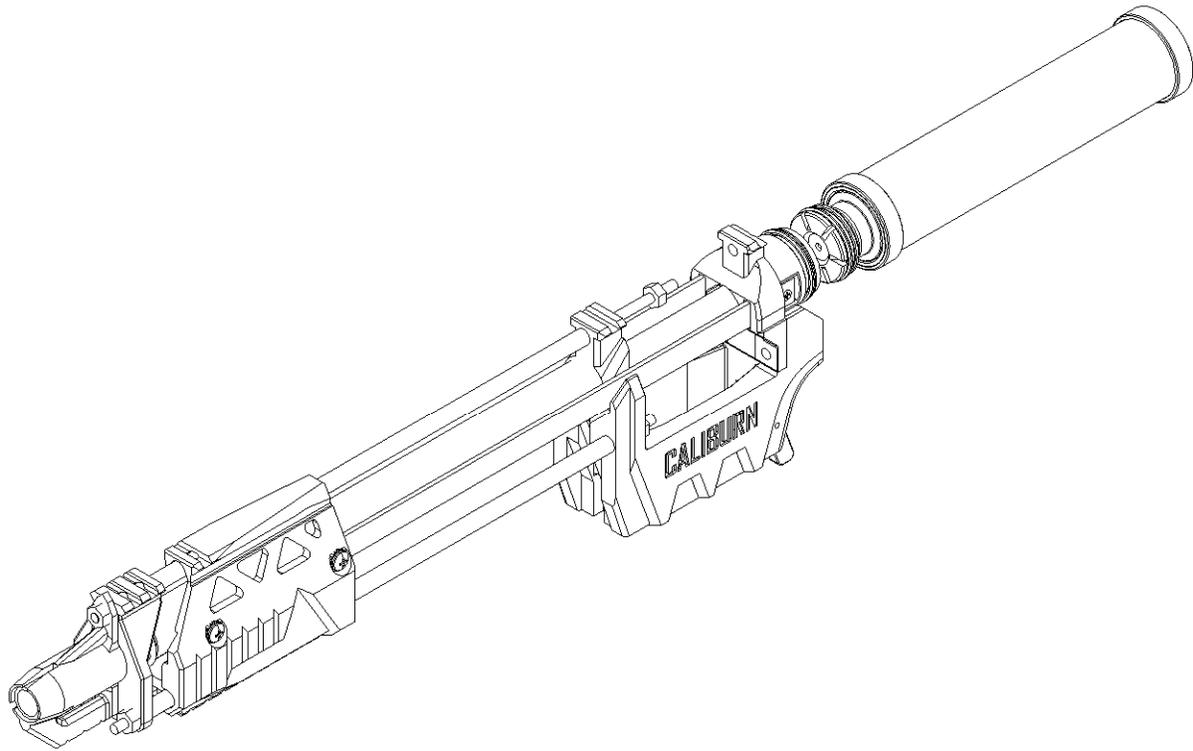
Slide the Plunger backwards into the Lubricated end of the Plunger Tube. Wiggle the Plunger Tube onto the O-Ring at the back end of the Ram Assembly.
