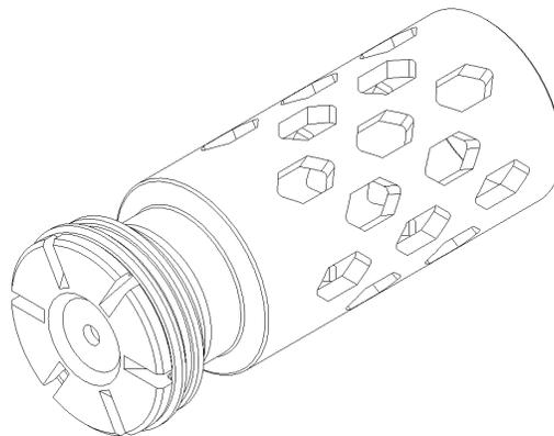
Add a Dash 123 O-Ring to the groove of the Plunger then set aside.
