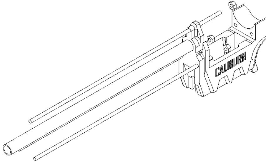
Slide two 13-inch length threaded rods into the lower holes at the front of the Mag Well. Slide one 14-inch length threaded rod into the upper hole at the front of the Mag Well. Add a hex nut to the inside end of each.
