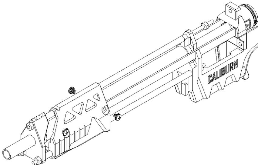
Slide the Foregrip forward. Secure the back half of the Foregrip with two more 1/4" length screws.
