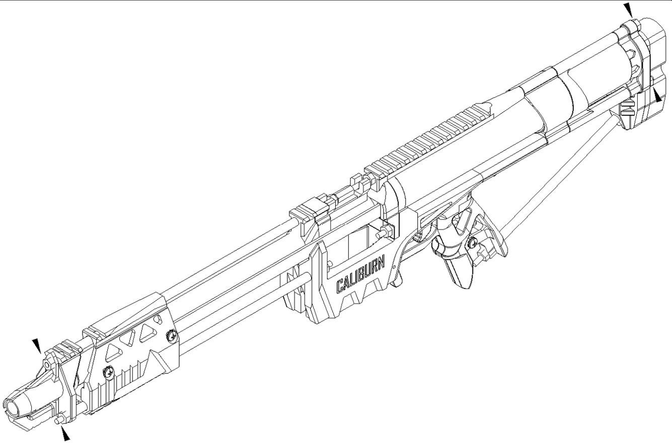
Use six Acorn Nuts to cover the exposed Threaded Rod ends at the front and back of the Blaster.
