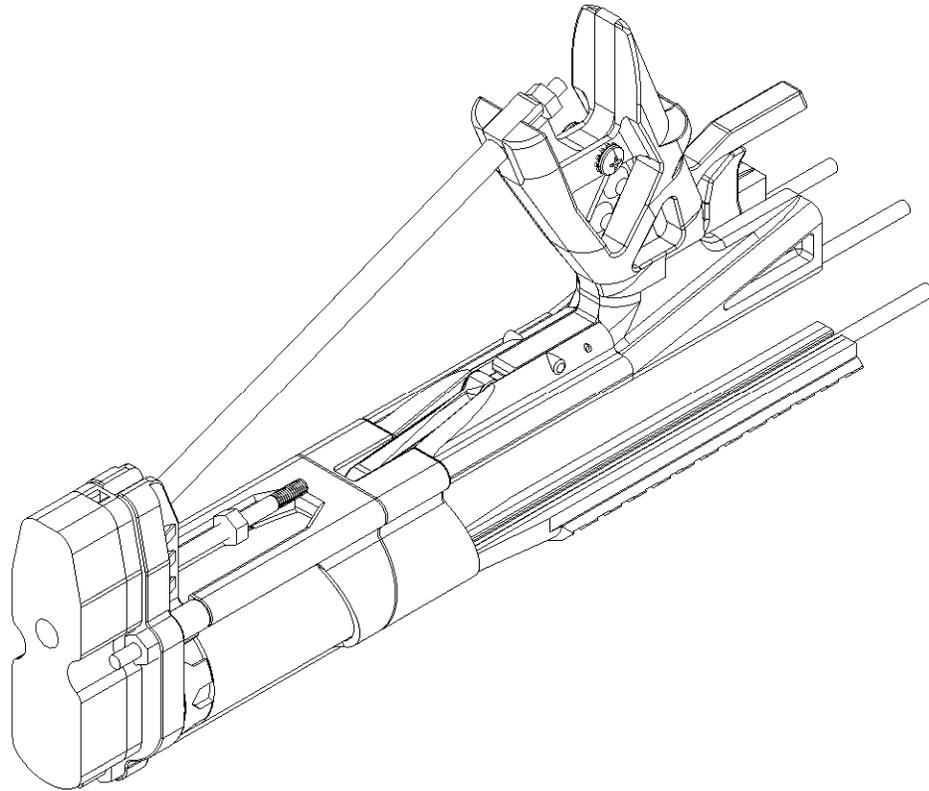
Add Buttplate to Butt. Secure with one or more Hex Nuts. Adjust to your desired spacing.
