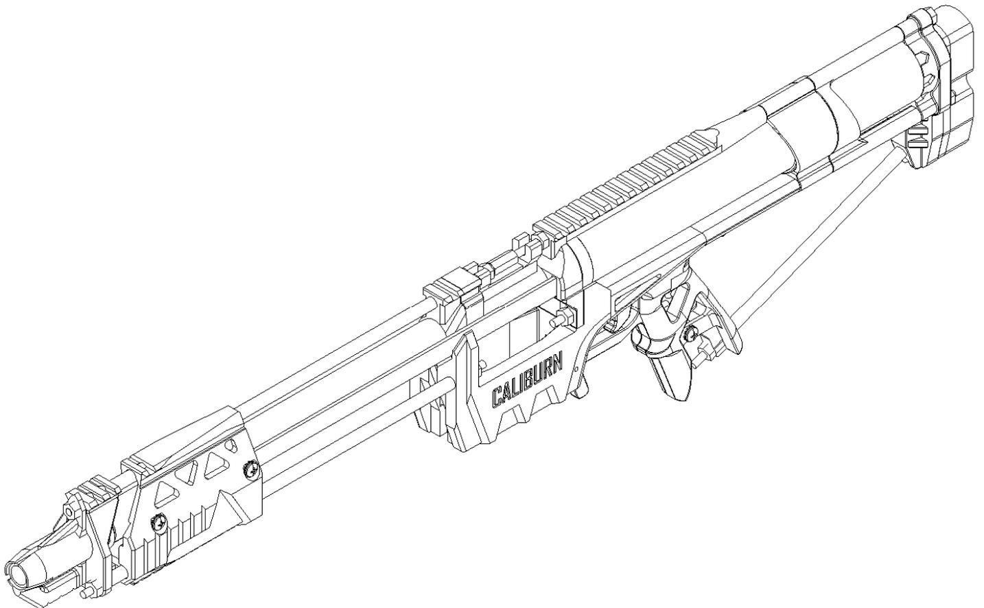
Install a Magazine loaded with darts and cycle the Foregrip back until the catch engages. Slide the foregrip all of the way forwards to chamber the dart in the top of the Magazine. You can load up to four darts into the barrel at a time if desired by cycling the Foregrip back and forth multiple times prior to pulling the Trigger.
