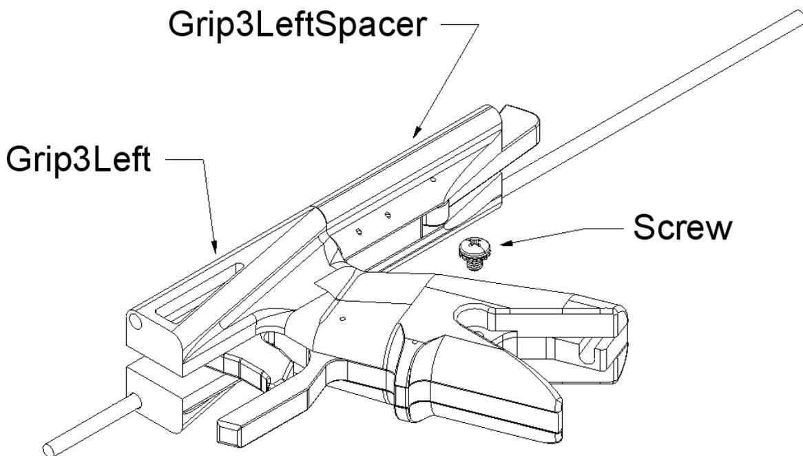
Slide Grip3Left and GripSpacerLeft onto the peg and secure it with a Screw.
