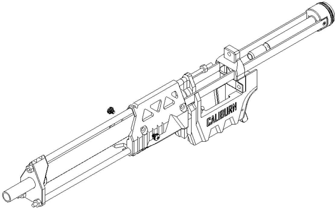
Slide the Foregrip back over the aluminum straps (Bolt Arms) until the threaded holes line up with the holes in the Foregrip. Secure them together at the front pair of holes using two 1/4" length screws. You may need to use a second screwdriver or other hand tool to push the aluminum against the inside of the Foregrip so the screw can reach it.
