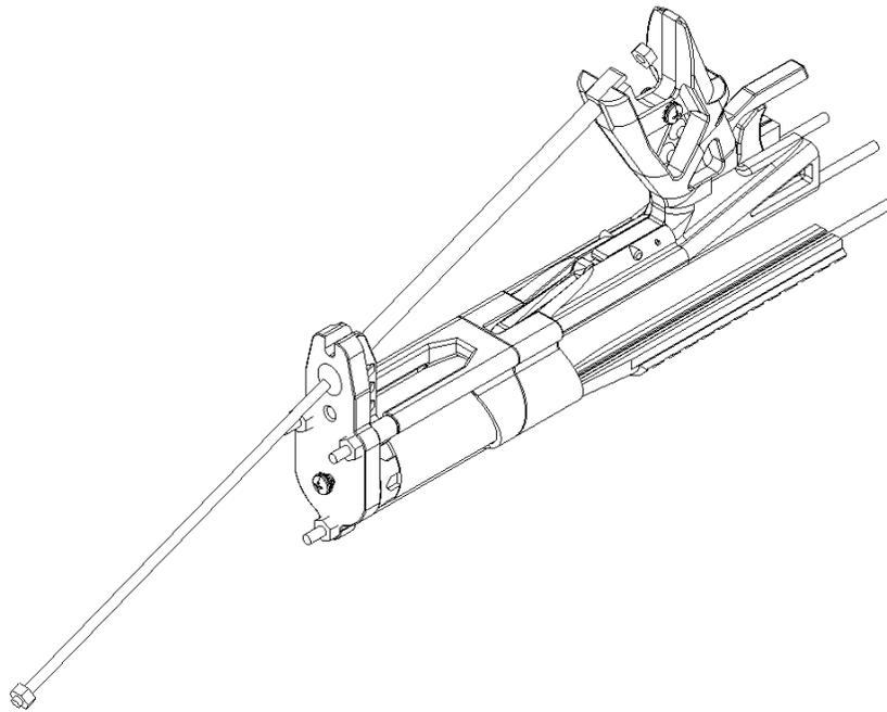
Wedge the 6" spacers inbetween the heel of the Grip and the front angled surface of the Butt. Add a Hex Nut to the very end of the 8" Threaded Rod and then slide it in through the counterbored hole in the Butt. Add a Hex Nut to the opposite end of the 8" Threaded Rod and tighten.
