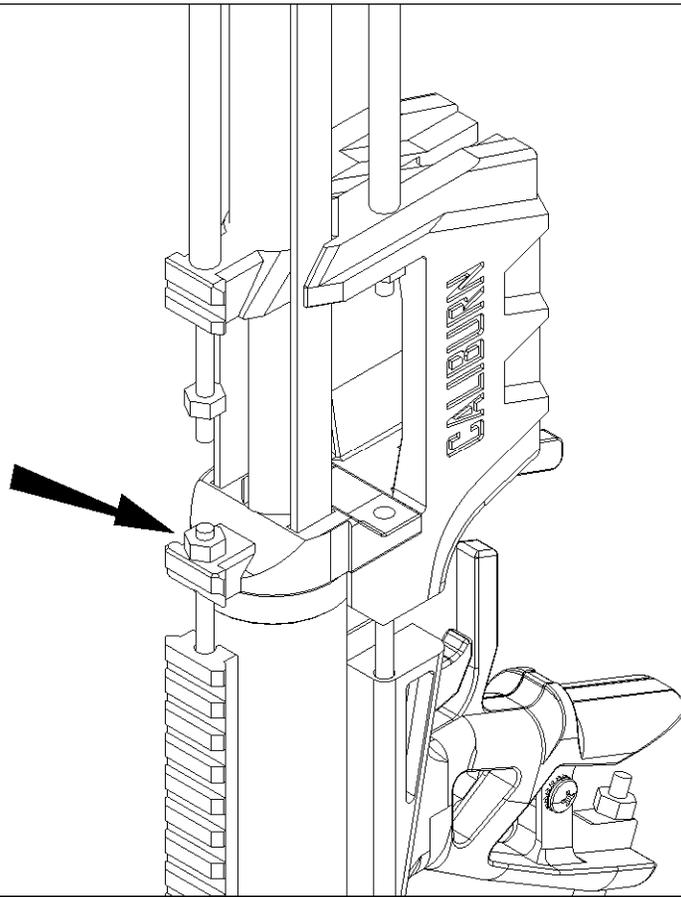
Feed the 14" Threaded Rod through the top hole of the Spreader and add a Hex Nut.
