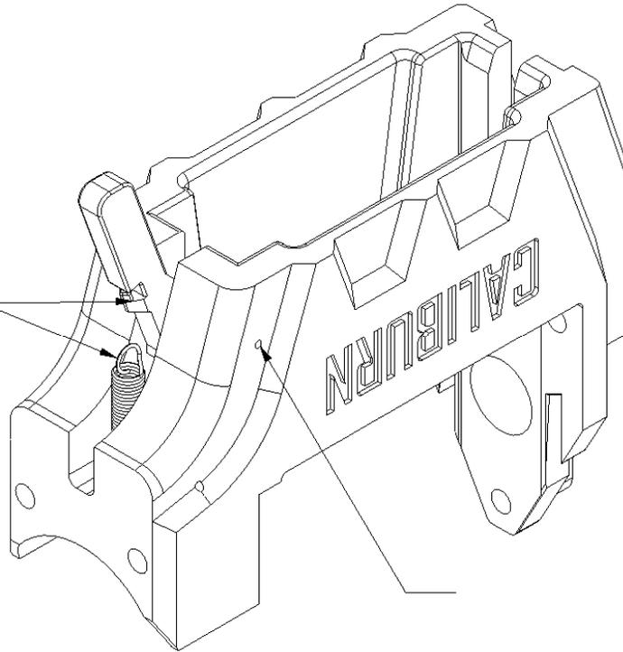
Pull the remaining loop of the Extension Spring onto the hook\peg on the Mag Release. Apply Super Glue to the indicated hole in left left side of the Mag Well or cut a very short section of Dash 123 O-Ring and plug the hole with it. If used, let the glue dry.
