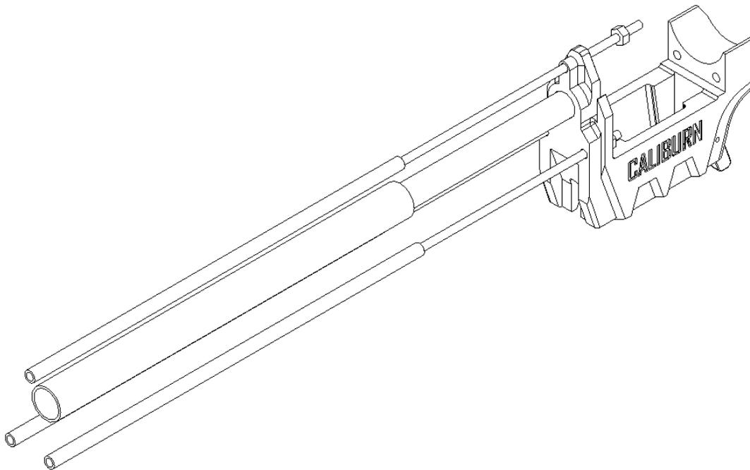
Slide three 11.25 inch length spacers onto the threaded rods. Also slide the Barrel Shroud over the barrel.
