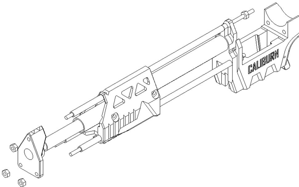
Slide the Muzzle onto the end of the Barrel, then fit the ends of the Threaded Rods through it. If included, slide the Muzzle Brake piece onto the barrel and upper threaded rod. Add three Hex Nuts and tighten the lower two.
