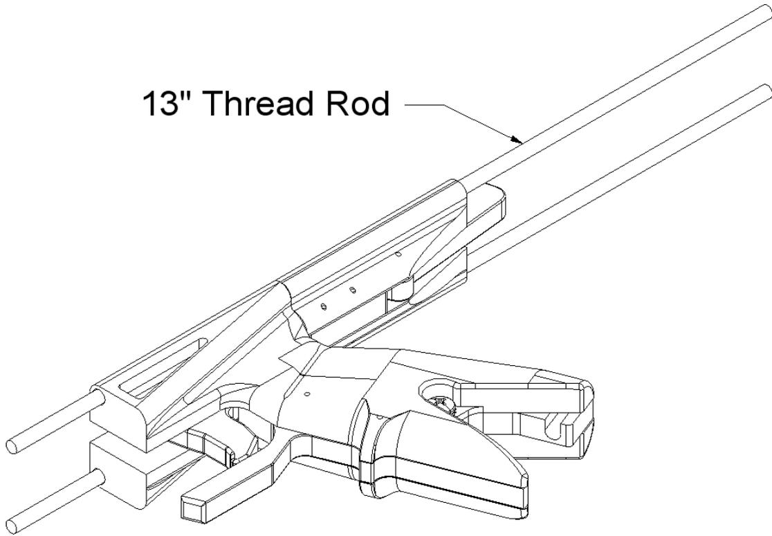
Slide a 13" Threaded Rod through Grip3Left and GripSpacerLeft
