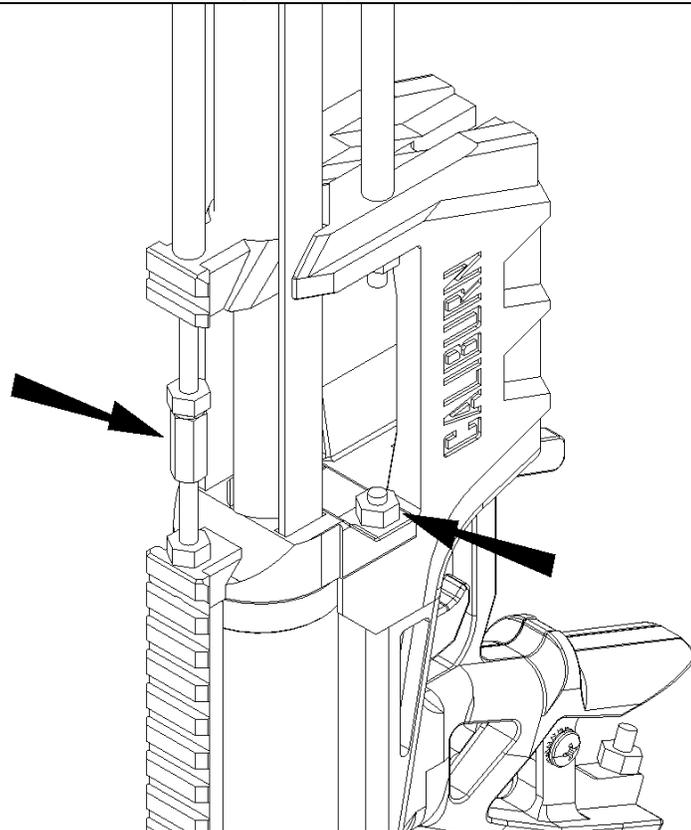
Also add the Coupling Nut to the 14" Threaded Rod, then guide the 13" Threaded Rods through the lower holes in Spreader and add Hex Nuts to those as well. Use the Coupling Nut to connect both 14" Threaded Rods together.
