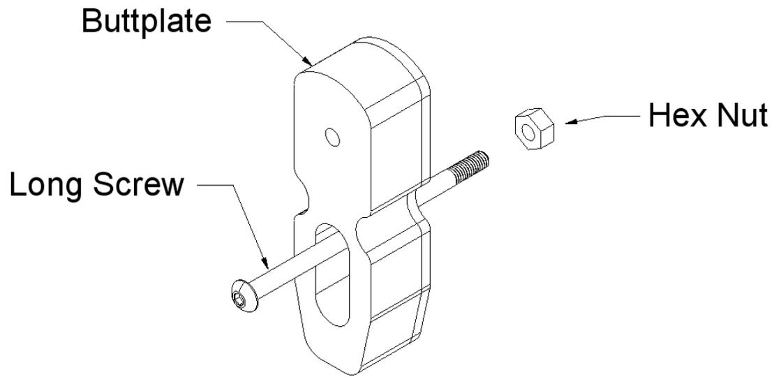
Add the LONG Screw THROUGH THE FOAM and use a Hex Nut to secure it to the Buttplate (or a Printed Alternative). Then Tighten the hex nut.
