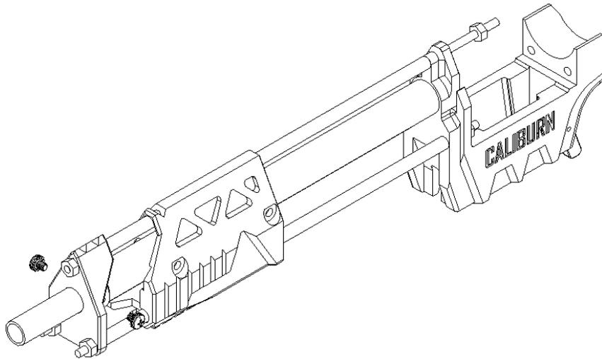
Confirm that the Barrel is still flush with the inside of the Mag Well. The Barrel can be secured using two 1/4" length screws if it has been tapped for them. Otherwise the barrel needs to be glued to the Muzzle using Super Glue or a strong epoxy such as Devon Plastic Weld or Plexus MA310.
