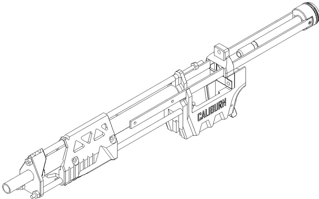
Install the Bolt Assembly by sliding it into the Mag Well from Above. Make sure that the Spreader part is ahead of the lip at the back of the Mag Well.
