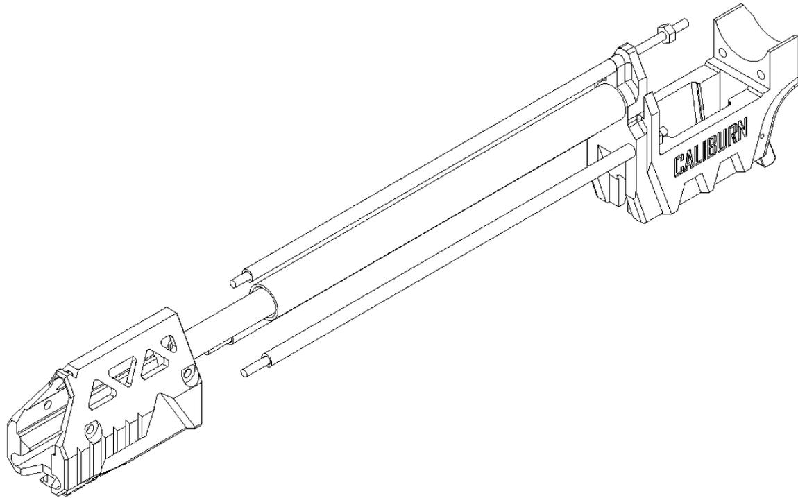
Slide the Foregrip over the now covered threaded rods and the barrel.
