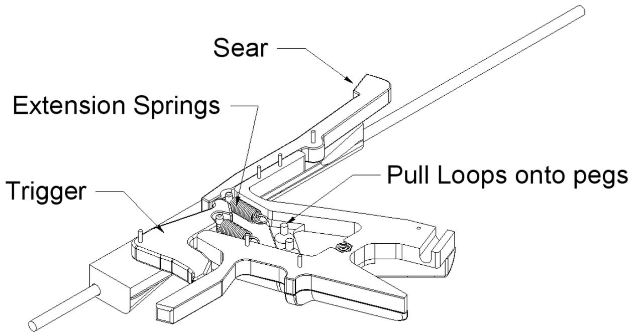
Slide the Sear and Trigger onto their pins. Put the loop of an Extension Springs onto the peg of each. Pull the opposite loop onto the pegs of TGuard2.
