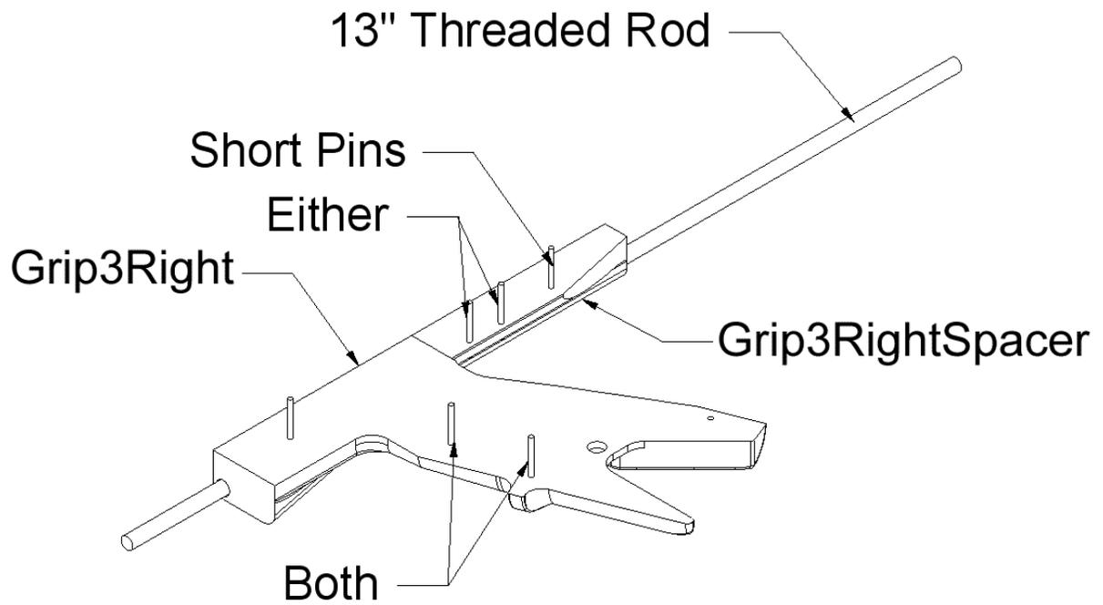
Slide the GripSpacerRight and Grip3Right onto a 13" Threaded Rod. Add Short Pins to most of the small holes as shown.
